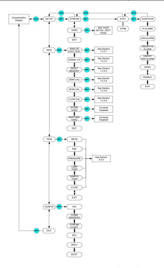
Figure 7-2: Front Panel Menu Diagram (Page 1)
